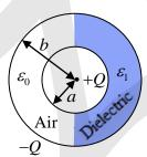
The electric field at a radial distance r from the center and between the shells (a < r < b)
