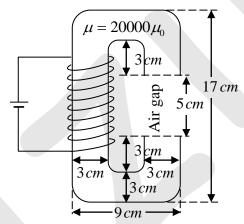
Ignoring the fringe fields, the magnitude of the magnetic field  $\vec{B}$  (in Tesla, rounded off to two decimal places) in the air-gap between the magnetic poles is \_\_\_\_\_.
